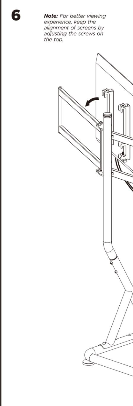
**Note:** For better viewing experience, keep the alignment of screens by adjusting the screws on the top.
