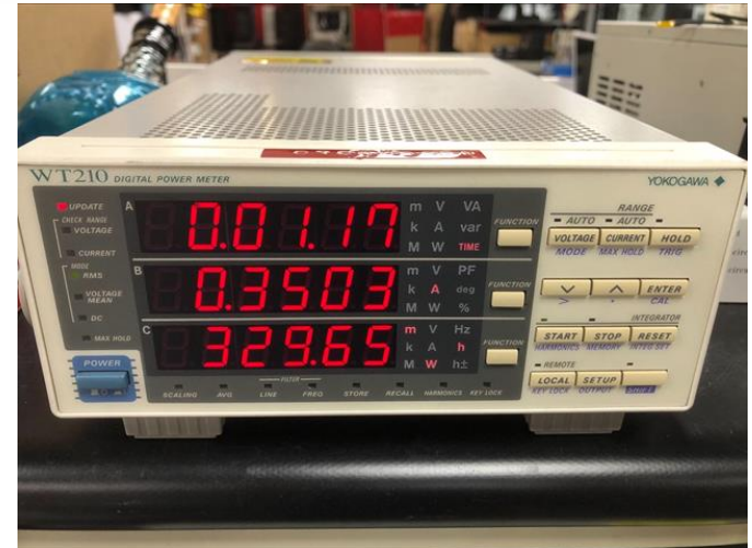
6. YOKOGAWA Power Meter WT210
