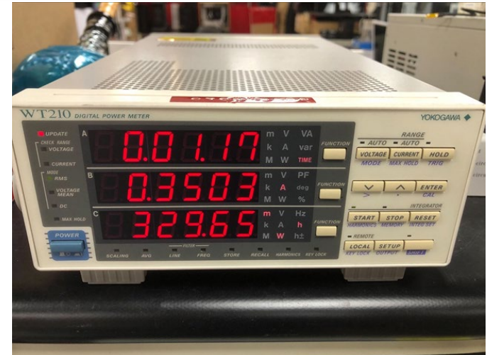
6. YOKOGAWA Power Meter WT210
