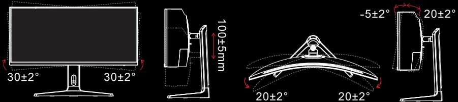
2.1 The screen can be adjusted by inclining forward and backward: however, the specific adjustment depends on the specific model of the device. Generally, it may be inclined  $5 \pm 2^\circ$  forward and  $15 \pm 2^\circ$  or  $20 \pm 2^\circ$  backward.
