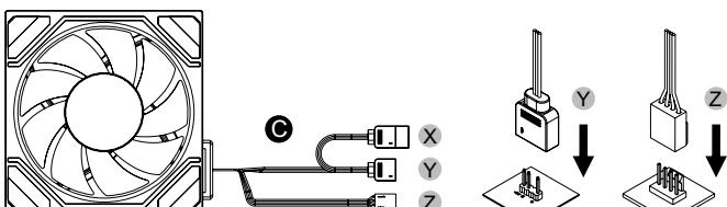
**CAUTION** Please power off the PC and check the Positive and Negative ends on the connector before connecting the cable to mainboard. Connecting the wrong end can damage the fans.
