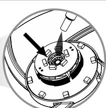
After replacing the fan blades several times, add the oil into the bearing (about 0.1ml)
