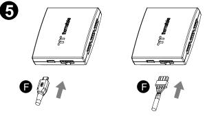
If you want to connect two or more controllers, you can sync the controllers with the bridge connector.
