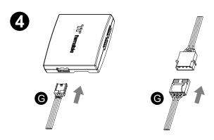
Connect the power cable to the 4pin Molex connecter and controller.
