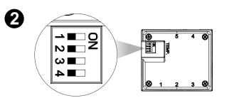
Set the DIP switch on the back side of the controller to assign the number of the controller
