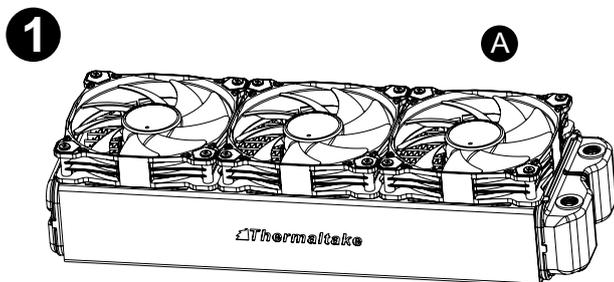
1 Install the fans properly onto the radiator
