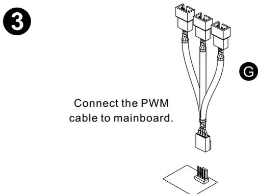
3 Connect the PWM cable to mainboard.
