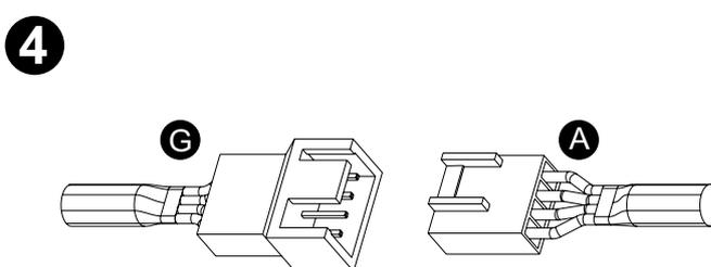
4 Connect the fan power cable to PWM cable
