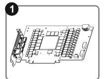
Disassemble the thermal module (cooler) of the graphics card and clean the thermal paste from the GPU
