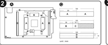
Cut the thermal pads to the dimensions listed and place them on the spots shown on the diagram.
