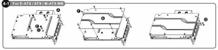
When installing the water block, carefully position the water block with the preinstalled standoffs on the graphics card.
