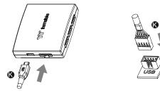
Connect the controller cable onto the motherboard (USB 2.0 9 pin) and controller.
