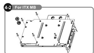
Caution: Please remove the backplate if the ITX MB interferes with the product during the installation process
