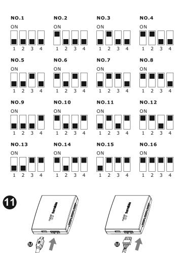
If you want to connect two or more controllers, you can sync the controllers with the bridge connector.
