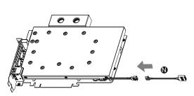
Connect the LED Cable on to the waterblock.
