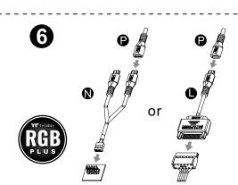
You could select one of the following ways of connections: 9pin USB 2.0(N): For power supply and TT RGB Plus 2.0 software control SATA(L): Only for power supply
