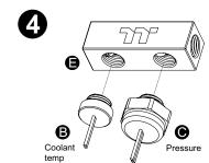
Install the liquid temperature sensor(B) and liquid pressure sensor (C) on the 4-way connector block(E)
