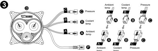
Connect the cables and connectors according to the corresponding labels
