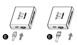
If you want to connect two or more connectors, you can use the bridge cable to connect the controllers.
