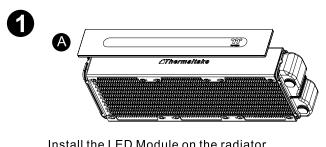
Install the LED Module on the radiator.
