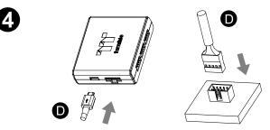
Connect the controller cable onto the mainboard (USB 2.0 9 pin) and controller.
