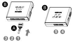
Connect the panel cable onto the controller.
