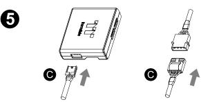
Connect the power cable to the 4pin Molex connecter and controller.
