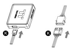
Connect the power cable to the 4pin Molex connecter and controller.
