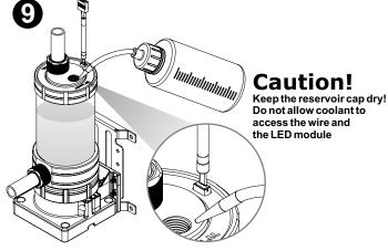
After adding the recommended coolant, remember to fill the reservoir to only 80% and leave the fill port cap off. This will help stabilize your internal loop pressure
