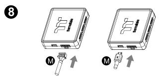
If you want to connect two or more connectors, you can use the bridge cable to connect the controllers.
