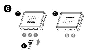
Connect the reservoir cable onto the controller.
