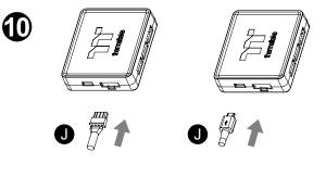
If you want to connect two or more connectors, you can use the bridge cable to connect the controllers.
