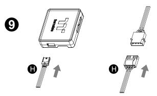
Connect the power cable to the 4pin Molex connecter and controller.
