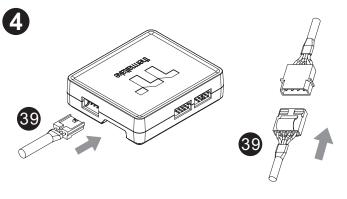
Connect the power cable to the 4pin Molex connecter and controller.
