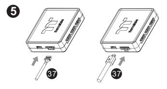
Connect the Bridge Cable to the Controller
