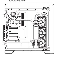
Fit the C-Pro fitting to the tube according to the order in the picture below, Install the tubes and tight the fitting caps.
