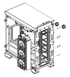
Attach the pump and reservoir into the chosen locations.
