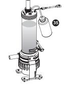
Place your PSU outside of the case and attach it to the pumps 4pin molex connector, turn on the power of PSU and make the rest of the system fills up.
