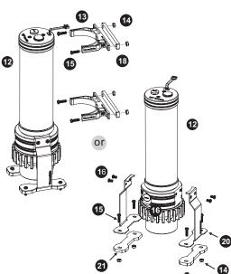
Attach fittings onto the pump and reservoir
