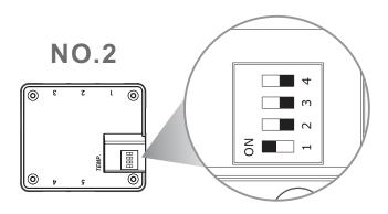
Set the DIP switch on the back side of the controller to assign the number of the controller.
