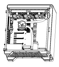
Measure the tube length based on the fitting, and make (cut) the tubes. The loop order: Radiator > Reservoir inlet
