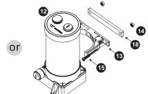
Attach fittings onto the pump and reservoir
