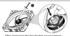
After replacing the fan blades several times, add the oil into the bearing (about 0.1ml)
