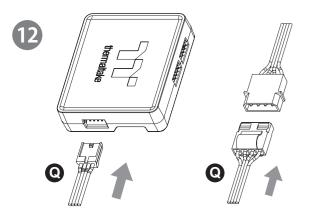
Connect the power cable to the 4pin Molex connecter and the controller.
