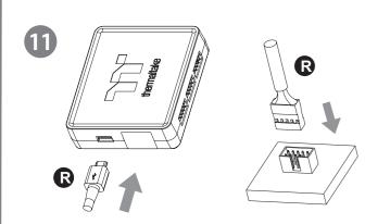
Connect the controller cable onto the mainboard (USB 2.0, 9 pin) and the controller.
