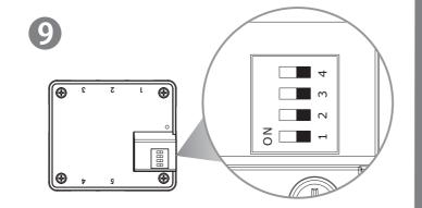
Set the DIP switch on the back side of the controller to assign the number of the controller
