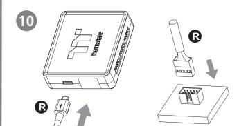
Connect the controller cable onto the mainboard (USB 2.0, 9 pin) and the controller.
