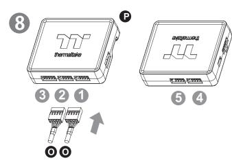
Connect the plug into the port in numerical order, start with plug one.
