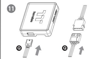
Connect the power cable to the 4pin Molex connecter and the controller.
