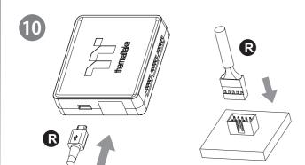
Connect the controller cable onto the mainboard (USB 2.0, 9 pin) and the controller.
