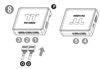
Connect the plug into the port in numerical order, start with plug one.
