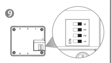
Set the DIP switch on the back side of the controller to assign the number of the controller
