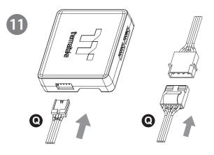
Connect the power cable to the 4pin Molex connecter and the controller.
