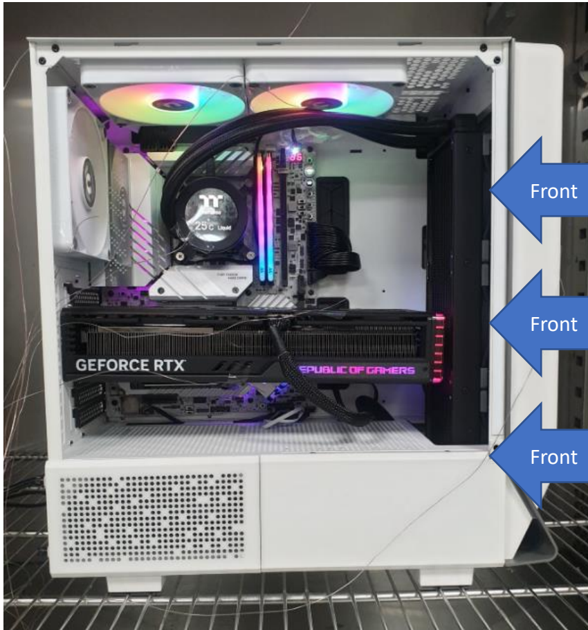
Cool Airflow Inlets (Active)
