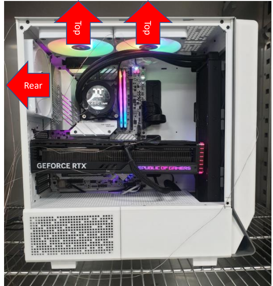
Hot Airflow Exhausts
