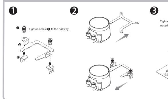
Tighten screw **①** again to ensure your waterblock is secure enough.
