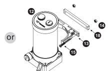
Attach fittings onto the pump and reservoir
