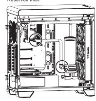
Fit the C-Pro fitting to the tube according to the order in the picture below, Install the tubes and tight the fitting caps.
