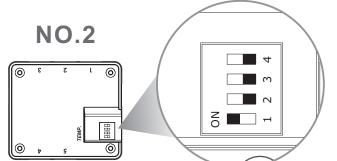
Set the DIP switch on the back side of the controller to assign the number of the controller.
