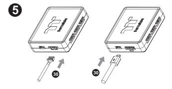
Connect the power cable to the 4pin Molex connecter and controller.
