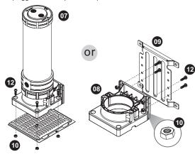
Attach fittings onto the pump and reservoir
