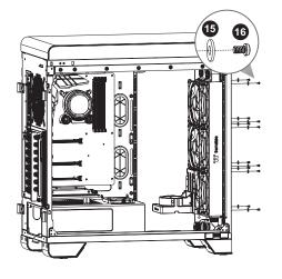
Attach the pump and reservoir into the chosen locations.
