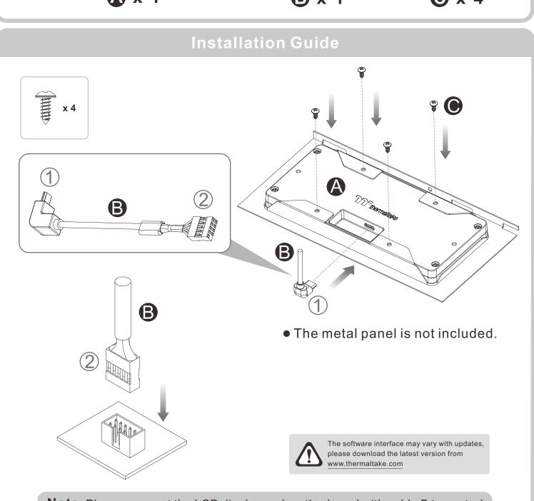
**Note**: Please connect the LCD display and motherboard with cable B to control the display with TT RGB PLUS Software.
