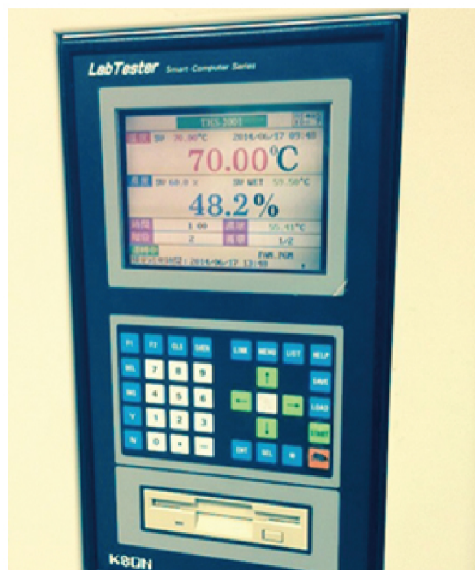
9.2 Batteries tested to extreme 70°C max and -20° low temperatures ranges.
