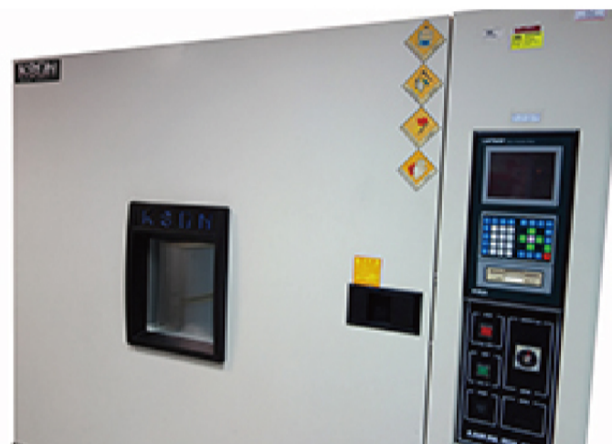
T1 Table 1 : Battery testing in high and low temperature ranges.
