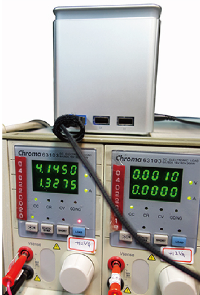
6.2 1A Output testing confirming 1.3A output.
