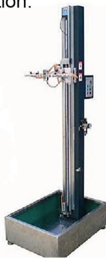
Portable battery bank drop testing machinery with adjustable height.
