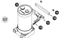
Attach fittings onto the pump and reservoir
