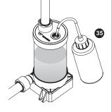
Place your PSU outside of the case and attach it to the pumps 4pin molex connector, turn on the power of PSU and make the rest of the system fills up.
