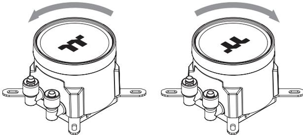
A rotatable LED cap built-in waterblock accommodates re-orienting the logo no matter the direction the cooler is installed
